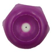
b. If you have access to an air compressor, aim the tip of the compressor gun at the white part of the nozzle and blow air inside. This will help to dislodge any debris blocking the nozzle orifice. Proceed to try the machine.
