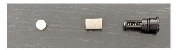
d. It is recommended to look inside the big pieces to make sure there are no debris inside. Remove any debris by running it the piece trough water, blowing it away with an air compressor or by removing it with a needle or a Q-tip. There is no risk to damage the piece with a needle.
