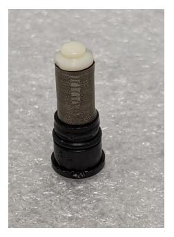
f. To reassemble the filter into its housing, simply insert it and firmly push it in with your fingers. You will hear a faint clicking sound once the filter is in its place.
